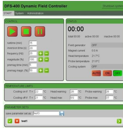
Figure 2. A field generator[2][3] (now fully digitalized and remotely controlled[net or mobile], produces a dynamic fiels, which moves every single magnetic particle – individually!- without generating particle heat! Relevant data are documented by the machine.
