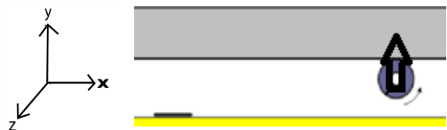
Fig. 6. This image shows, that the magnetic field \vec{B} , established by the field generator (yellow area), is concentrated on top of the washer. This top area is saturated (arrow) meaning, that all the field lines are in parallel and all the spins \vec{m} in the washer are in line with this field.
